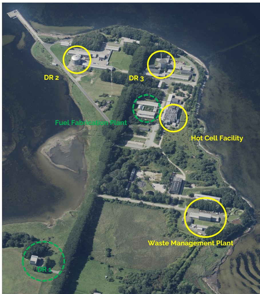
Figure 2: Aerial photo of the Risø Peninsula. All Danish nuclear facilities are located on the Risø site. Yellow circles indicate nuclear facilities under decommissioning. Green circles indicate nuclear facilities that are fully decommissioned and released from regulatory control.
