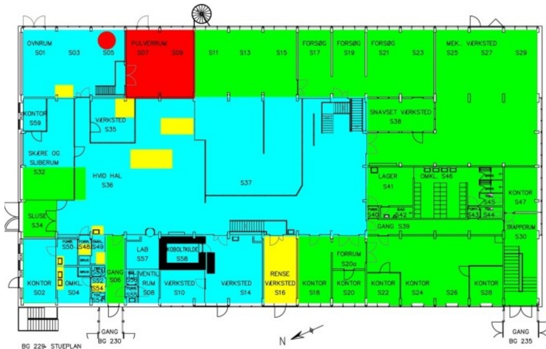
Figure 10. Radiological classification of ground level areas in the Fuel Fabrication Facility as of 2013: Red – Contaminated. Yellow – Probably contaminated, Blue – Not contaminated, reassurance measurements required, Green – Not contaminated, reassurance measurements not required.
