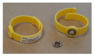
The dosimeter element itself, of the Harshaw DXTRAD<sup>™</sup>-type, is a small metal ring with polyimide (Kapton<sup>™</sup>) and a thin layer of radiation-sensitive thermoluminescent lithium fluoride powder. The element is covered by a flattened plastic dome with a thin window on the outside. The elements have individual barcodes and are manufactured by Harshaw<sup>™</sup>, part of Thermo Fisher Scientific.
