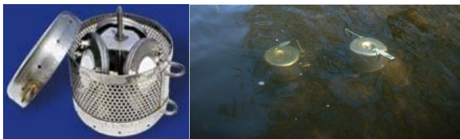
Fig. 3. Polar Organic Chemical Integrative Sampling (POCIS).
