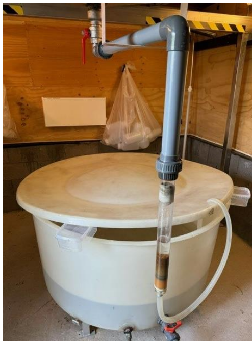
Figure 9: Rain tank with the ion exchange resin
