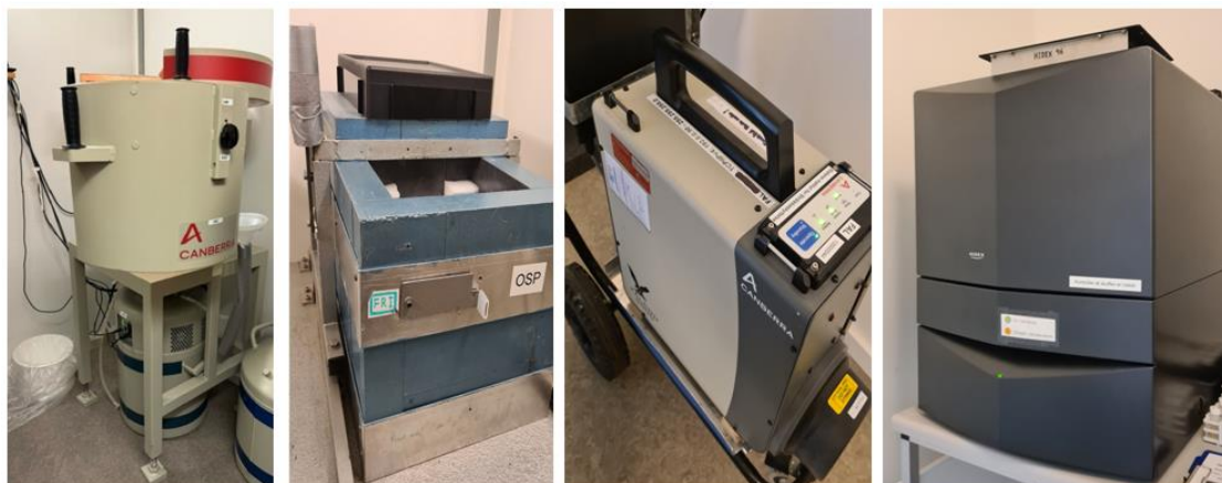
Figure 18: Counting equipment at the DHA/RP radionuclide identification and quantification laboratory (Mirion HPGe-detector, NaI-detector, portable Mirion HPGe-detector and Liquid scintillation counter-Hidex 300SL)
