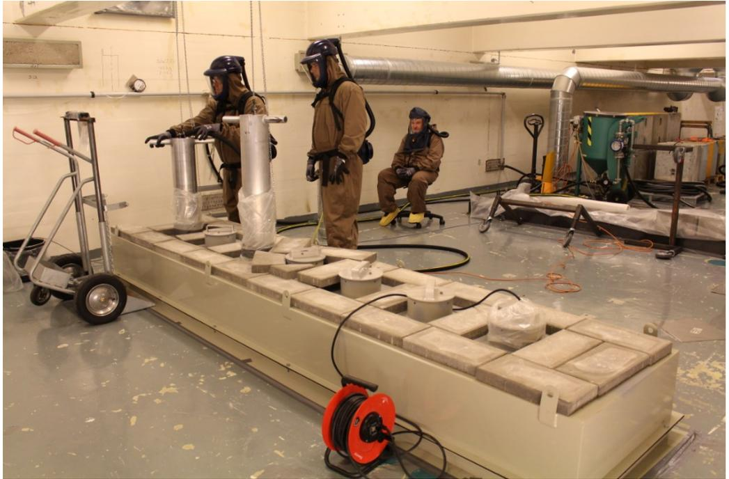
Figure 17: The complete setup of the steel grit blasting. The blowing nozzle is placed in the first hole and the camera in the third.
