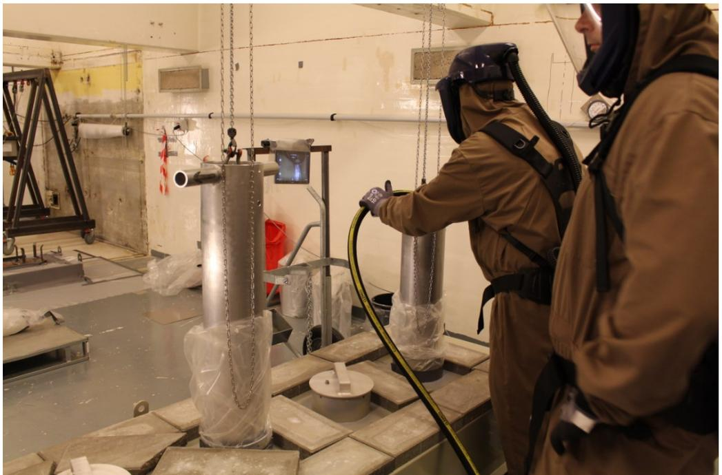
Figure 18: The operator controls the blowing nozzle and at the same time keeps an eye on the media blowing through the camera surveillance.
