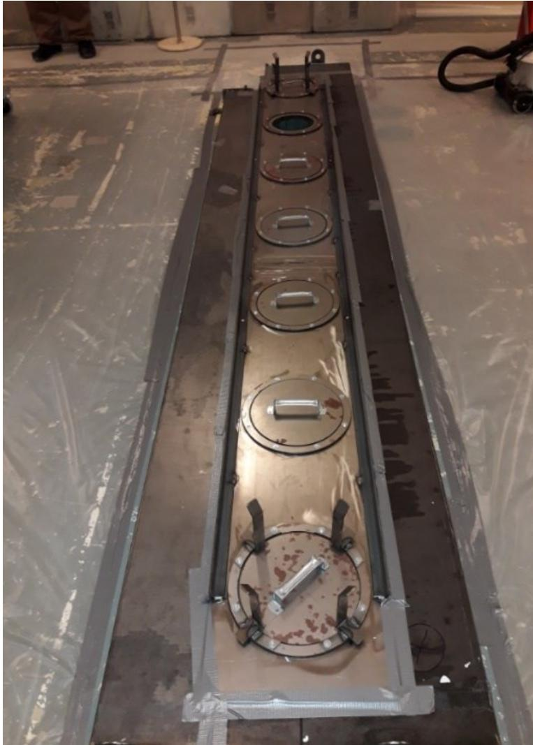
Figure 15: Dummy shutter housing after modification
