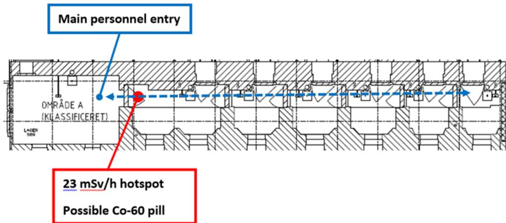
Figure 19: Hotspot location at the entry to the hot cells
